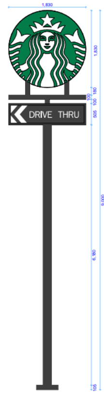
Proposed sign (not to scale: 9m high) The logo & DRIVE THRU box are internally lit.
