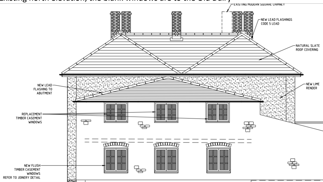
Proposed north elevation with Dairy windows replaced
