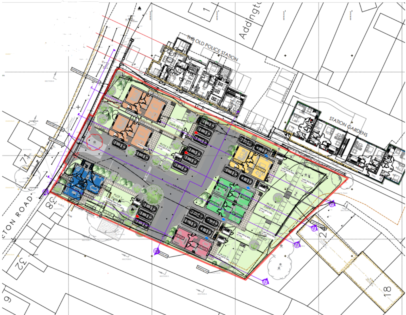
Amended Site plan with neighbouring properties clockwise from bottom left) – 32-38 Moreton Road (terrace of cottages - NDHA); 71 Moreton Road (Brae Lodge); site with permission for 12 houses; Old Police Station (Listed Building converted to flats); Station Gardens (block of 8 modern flats); 18-24 Mary MacManus Drive (bungalows: Sheltered Housing)
