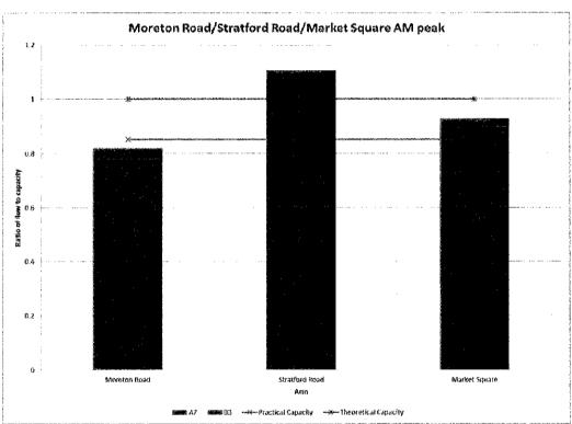
The results of the analysis show that in the **base situation** (A7), with consented and allocated developments, the Stratford Road, Bridge Street and West Street approaches to the junctions will be over capacity with significant queuing in the evening peak hour.
