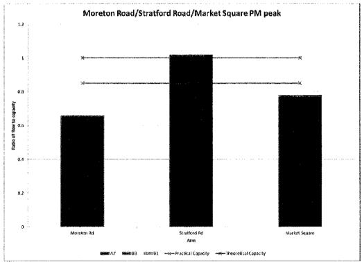
The modelling of Scenario A7 and B3 shows that in the AM and PM peak, the RFCs would only increase marginally on all approaches when the Phase 3 development flows are added. The cumulative impact of this development and the allocated sites in the BNDP on the mini roundabout junctions within the town centre are however significant.
